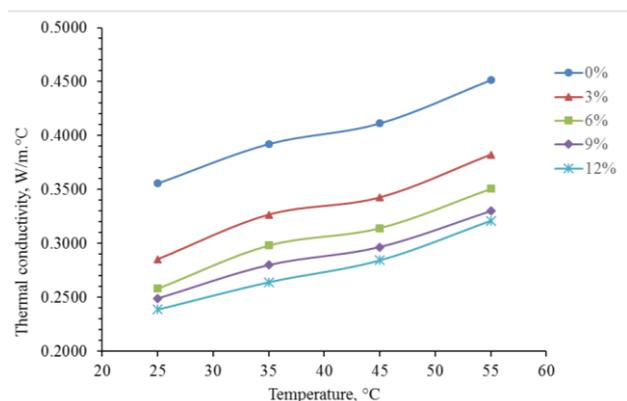
Fig. 3 Relationship between thermal conductivity and temperatures at different pistachio shells particles volume fractions
