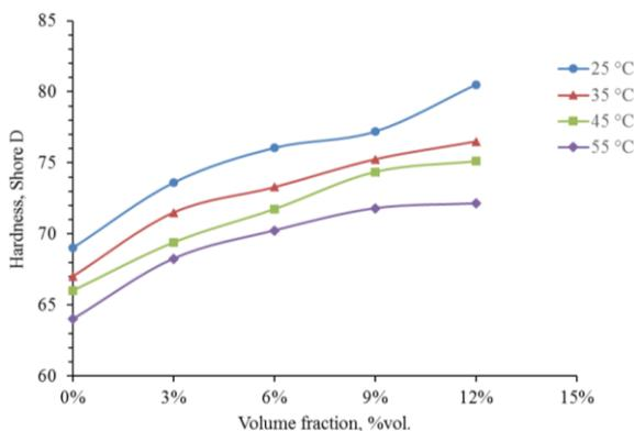
Fig. 2 Relationship between hardness and pistachio shells volume fraction at different temperatures
