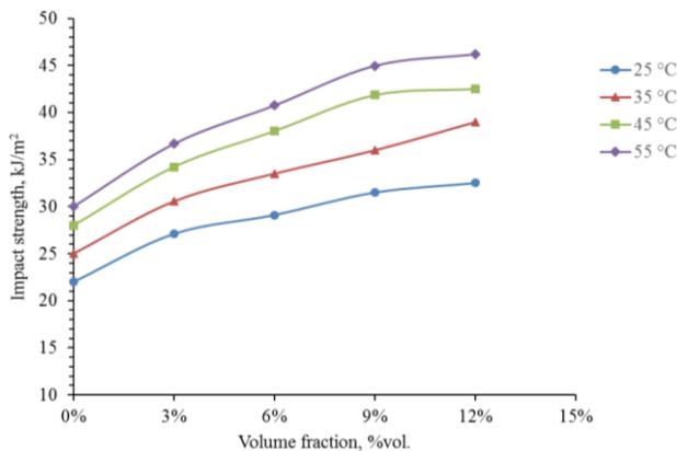
Fig. 1. Relationship between impact strength and temperatures at different pistachio shells volume fractions of the BEP materials used
